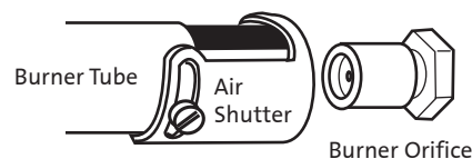
Figure 12. Burner Orifice and Air Shutter. Shutter is shown in the fully open position.
